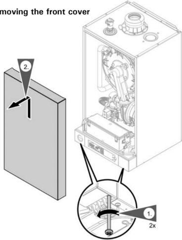
1. Loosen retaining screws, screws are captive and do not need to be fully removed.
