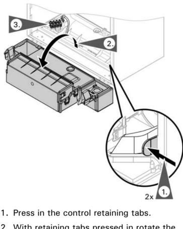
1. Press in the control retaining tabs.
