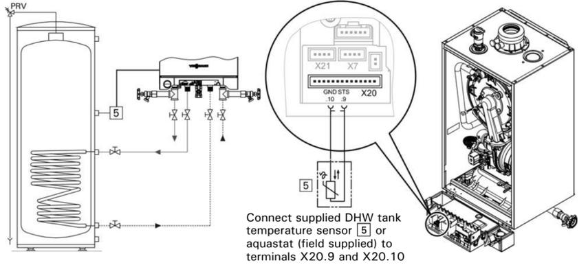
Connect supplied DHW tank temperature sensor [5] or aquastat (field supplied) to terminals X20.9 and X20.10
