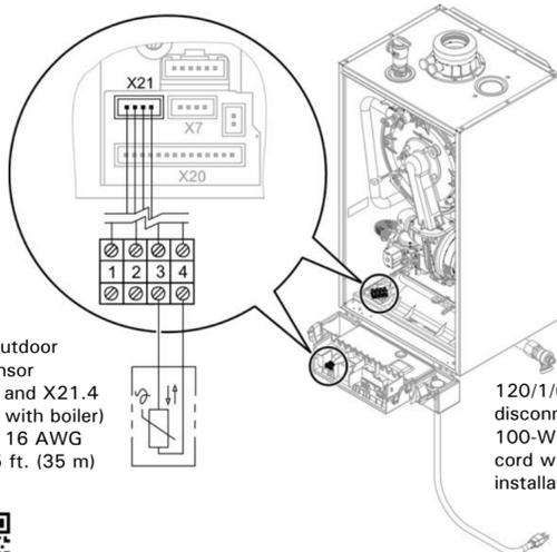
Connection to Outdoor Temperature Sensor terminals X21.3 and X21.4 (sensor supplied with boiler)
