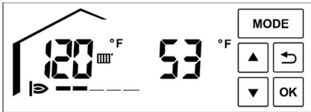
Left side of the display shows current boiler water temperature. Right side displays current outdoor temperature.
